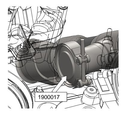
Place the cap using v band clamp on the EGR port and thighten the v-band clamp nut 6 N-m (53 lb-in)
