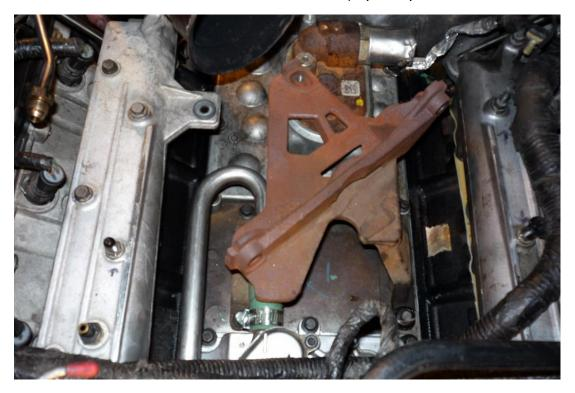
Install turbo oil drain with new O-rings.
