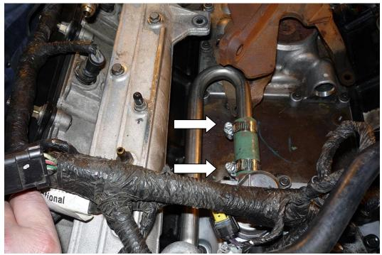
two (2) steps. 1 - Starting at the front and working towards the back, tighten bolts to 50 inch lbs of torque, then 2 - again starting at the front and working toward the back, tighten bolts to 100 inch lbs. Then install, at the front of the intake, two (2) 15mm bolts and torque to 23 ft lbs and one (1) 10mm bolt to 18 ft lbs. Install the silicone coolant hose with two (2) HS10 hose clamps (*P/N 1453113*).
