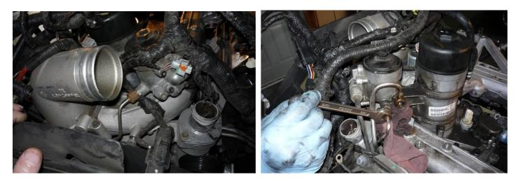
Disconnect the fuel filter wiring connectors and fuel lines then remove fuel filter housing.
