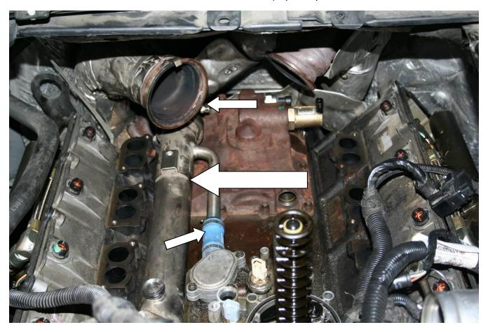
Remove the EGR cooler by disconnecting the clamp at the exhaust feed pipe then remove the coolant hose by first cutting the front clamp then twisting to align the release tab and pulling (you may have to spread the tab with a small pick or screwdriver).
