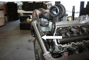
Loosen the driver's side exhaust feed pipe hardware at the manifold.
