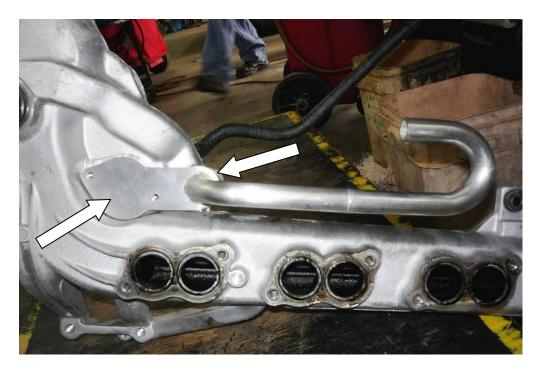
Install newly supplied (#1400283) O-ring on the EGR Cooler Bypass Pipe then install pipe into the bottom of the intake. Install supplied oring **(#1900016)** into the blocker plate (1900010-V2) and install with the cooler bypass pipe over the exhaust port and tighten to 100 inch lbs of torque. (NOTE: This plate secures the
