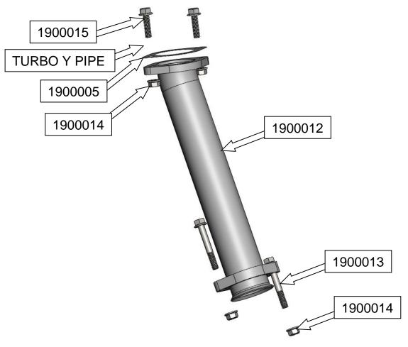
Install the newly supplied passenger side feed pipe using the supplied hardware. Install the supplied gasket (#1900005) on the top side of the pipe. Tighten the four nuts (13 mm socket) to 20 ft lbs. Reinstall the heat shield with new rivets if applicable. Install the lower mounting hardware at the manifold leaving loose.
